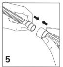
Connect the short tube to the flow generator's air tubing.
