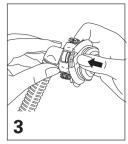
Push pillows firmly into frame. Ensure top and bottom retention tabs slot into place.
